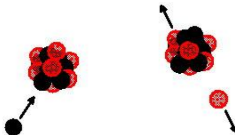
Before collision of neutron (black) with nitrogen-14 nucleus, 7 protons (red) and 7 neutrons. After collision, neutron is captured and proton is ejected, resulting in carbon-14 with 6 protons and 8 neutrons. (Fig.1)
