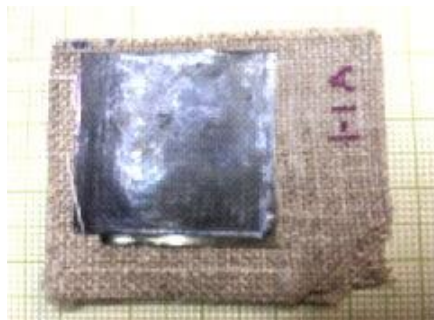
Figure 8. Four lead foils on top of five linen samples. (1-centimeter graph paper for scale reference.)
