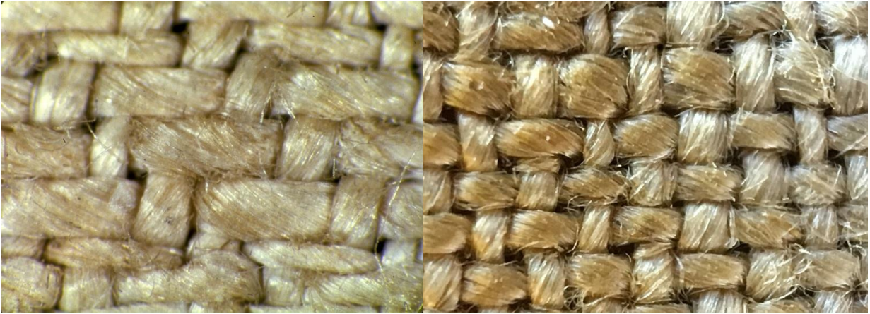
Figure 11. Comparison of Shroud image near foot (left) and proton irradiated modern linen (right). At the edge of proton beam where density of protons declines, it matches the character of what is seen on the Shroud. The Shroud image has a much higher magnification.
